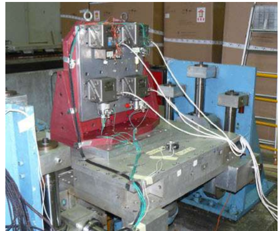
Delta Switches being seismically tested at the SOPEMEA test facility in France to the RCC-E seismic spectra
